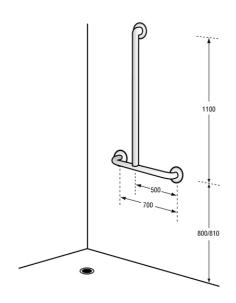
This product is AS1428.1 compliant (accessible compliant) when installed in accordance with the guidelines.
